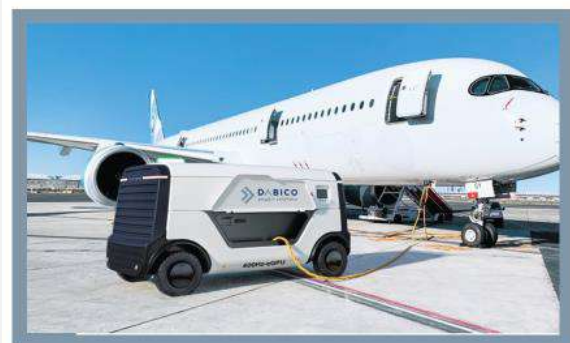
Dabico's 400Hz battery-powered ground power unit for aircraft. Photo owner: Dabico Airport Solutions
