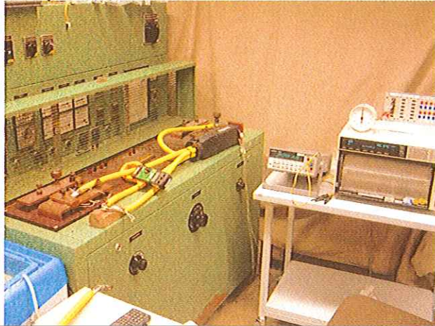
Foto 1.3 / Picture 1.3 Messung Isolationswiderstand Measurement Insulation resistance
