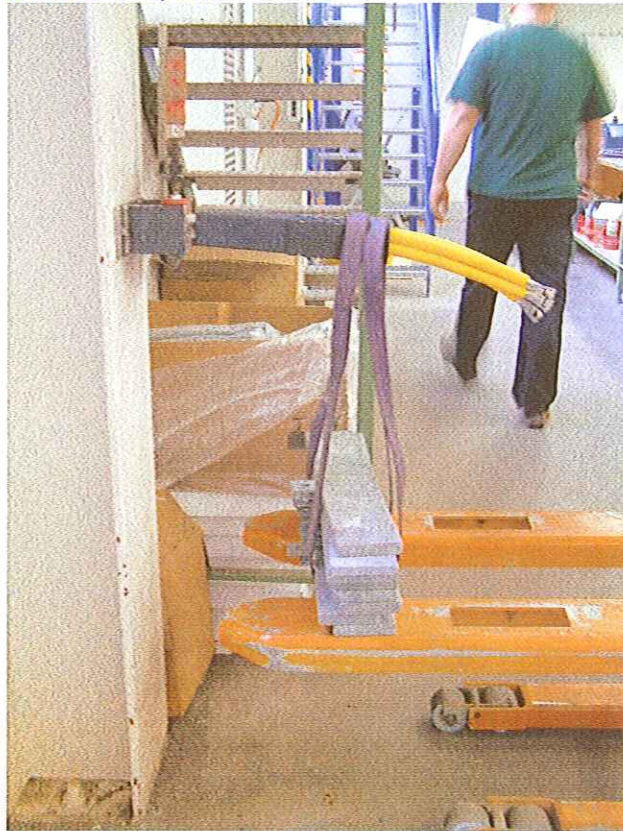
Foto 8.5 / Picture 8.5 Statisch Querlast, Start Side load test, start
